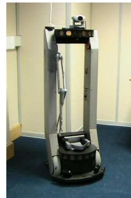
Figure 1: The PeopleBot™ robot used in the experiments.
