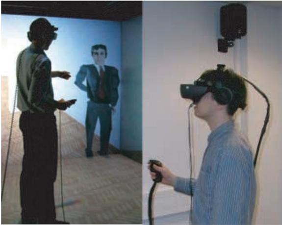
**Figure 7:** *Left - Participant in the CAVE™-like ReaCTor system. Right - Participant in the Head-Mounted Display.*
